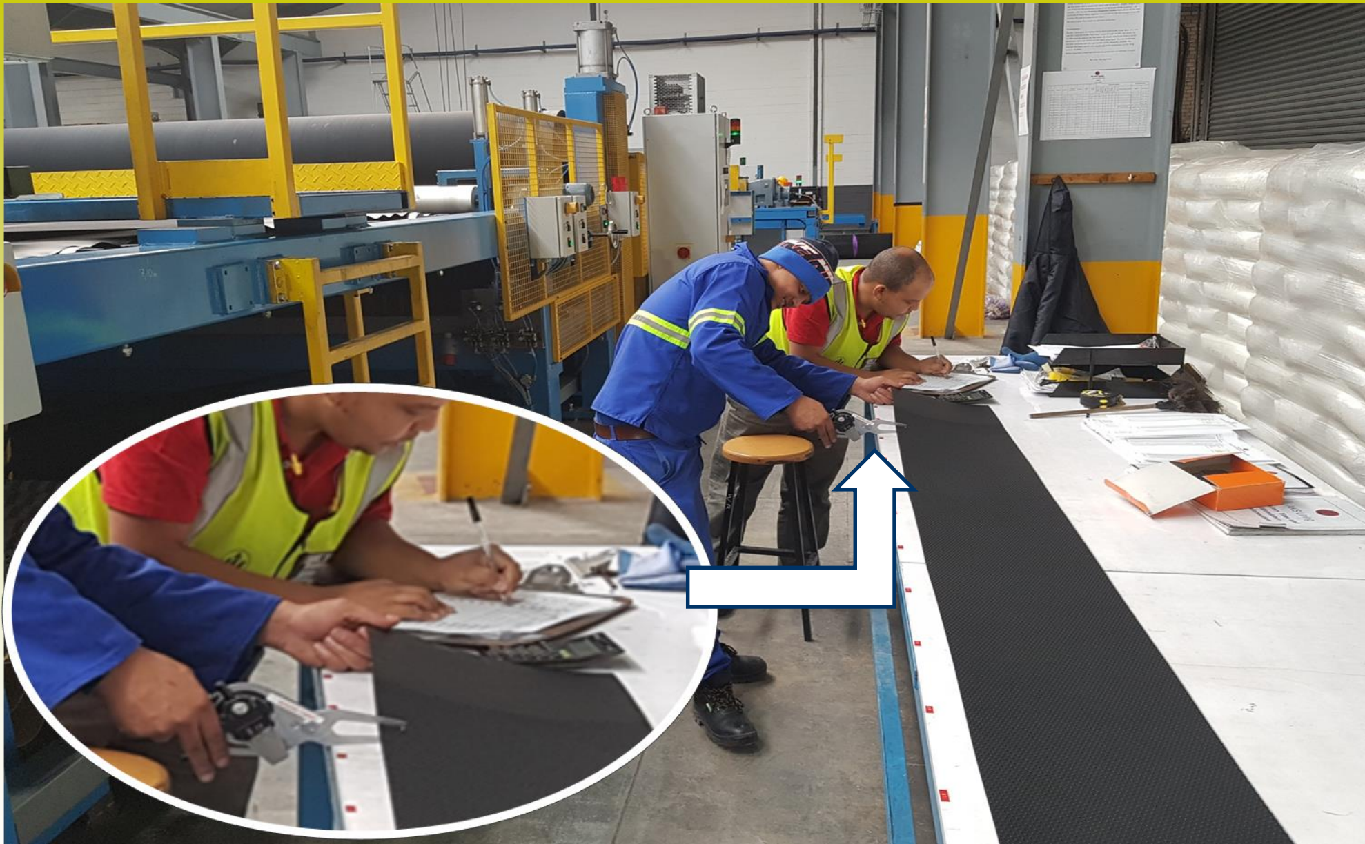
Thickness control 36 zones = 36 checks. GRI-GM13 = 10 checks.
