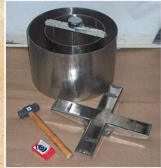
**QA/QC – On site permeability testing using double ring infiltrometer testing apparatus**
