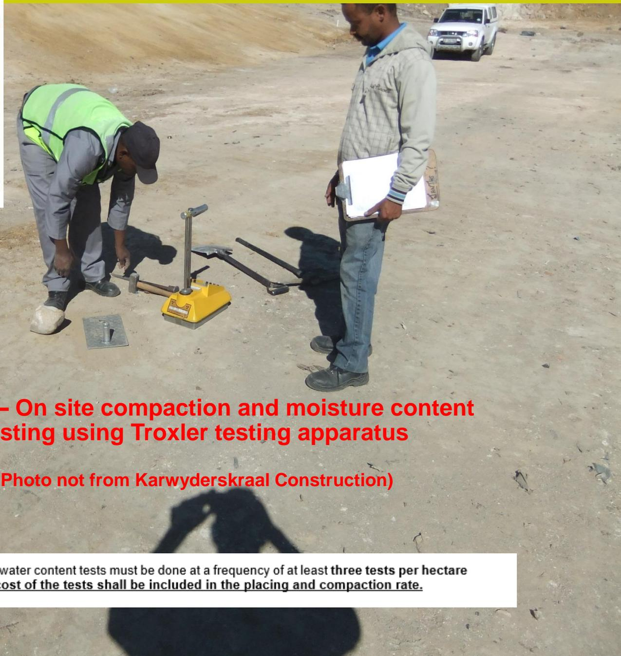
**QA/QC – On site compaction and moisture content testing using Troxler testing apparatus**
